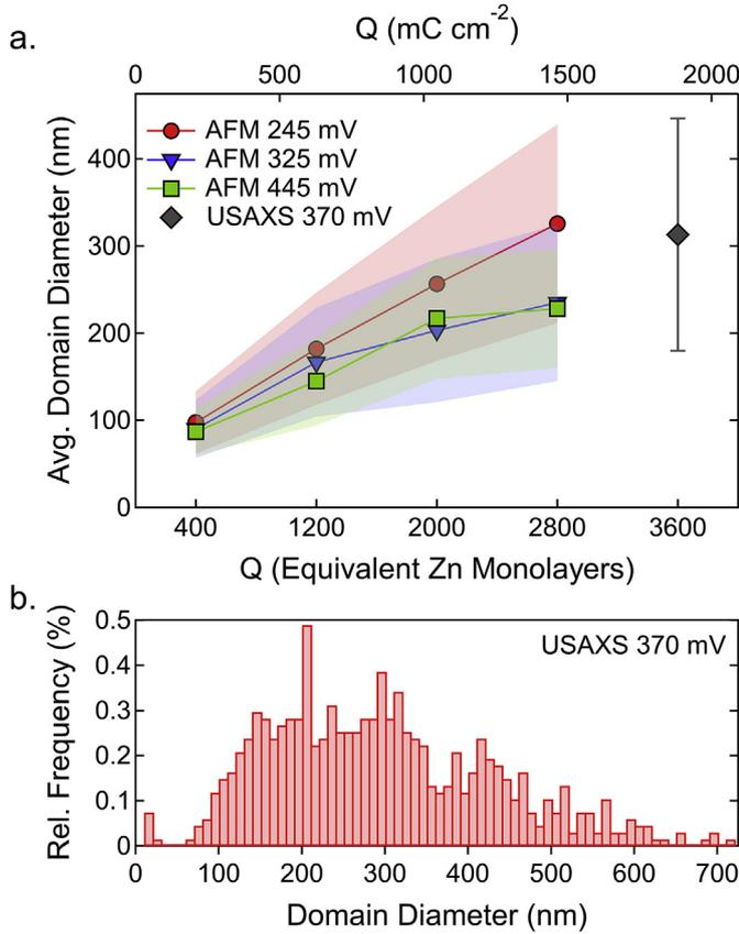
**Fig. 7.** (a) Average Zn domain diameters measured from *in situ* AFM imaging (AFM 245 mV, AFM 325 mV, and AFM 445 mV) and SEM images obtained from the Zn surface after deposition within the USAXS cell (USAXS 370 mV) plotted against the amount of charge passed. The shaded regions and horizontal bars represent the standard deviation range for the measured domain diameters. (b) Histogram showing the relative frequency of the domain diameters for the USAXS 370 mV data.
