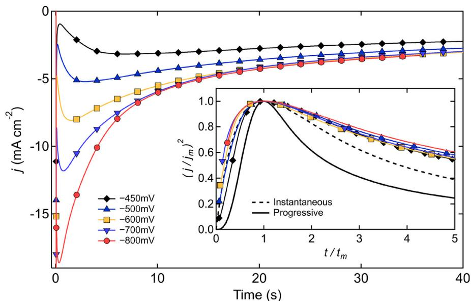
**Fig. 3.** Chronoamperograms of a Pt electrode in  $0.34 \text{ mol kg}^{-1} \text{ Zn(TfO)}_2/\text{BMIm TfO}$  at  $25^\circ \text{C}$  for various applied potentials vs. Zn wire. The inset figure shows the data normalized to the maximum current density and the corresponding time where the solid and dashed lines correspond to the theoretical models for progressive and instantaneous nucleation.
