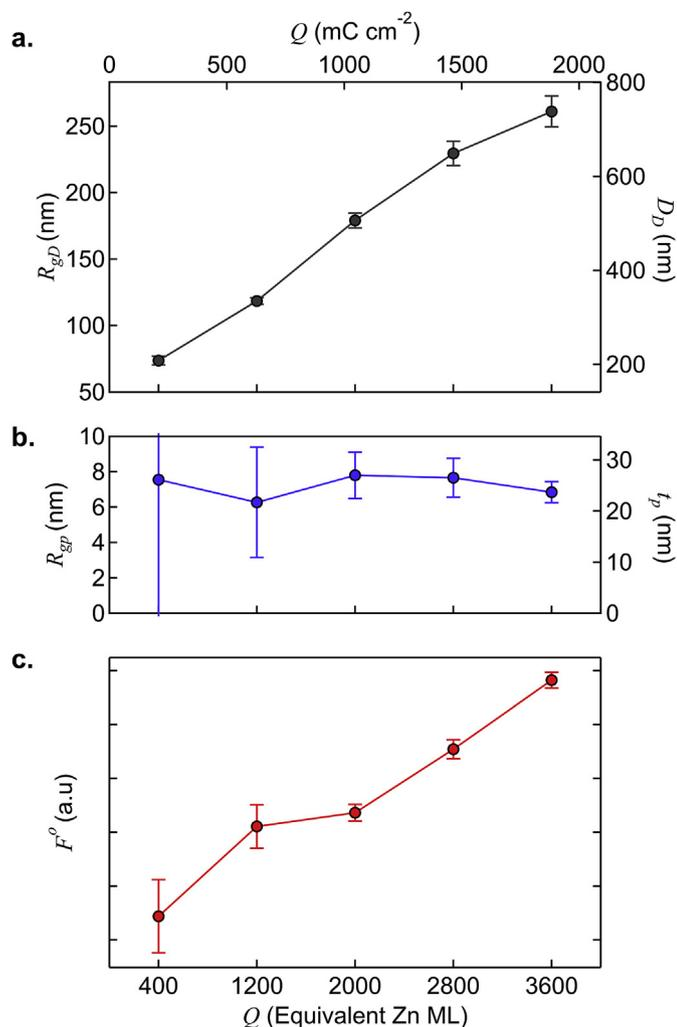
**Fig. 12.** Unified model fits of the radii of gyration from the (a) domains and the (b) zinc plates, along with (c) the degree of plate coalescence,  $F^o$ , as a function of the zinc monolayers of charge passed. The horizontal bars represent the standard errors obtained from the least-squares linear fitting of the data within the Irena package for Igor pro.
