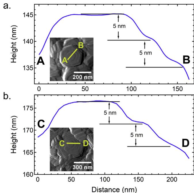
**Fig. 9.** Examples of AFM height profiles along zinc crystallite layers for the same zinc domain during deposition within  $0.34 \text{ mol kg}^{-1} \text{ Zn(TfO)}_2/\text{BMIm TfO}$  at a reducing potential of  $-245 \text{ mV vs. } E_{\text{CO}}$  growth after (a) 1200 Zn ML ( $627.6 \text{ mC cm}^{-2}$ ), and (b) 2000 Zn ML ( $1064.0 \text{ mC cm}^{-2}$ ) of charge passed. The letters designate the direction of the height profile.
