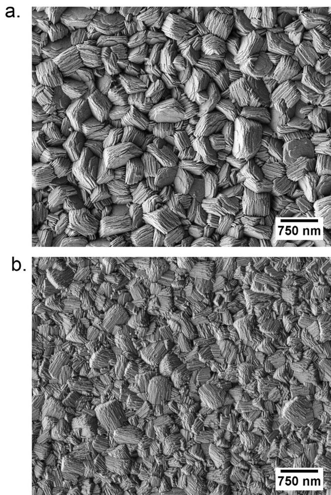
**Fig. 5.** SEM image of the zinc surface after deposition in  $0.34 \text{ mol kg}^{-1} \text{ Zn(TfO)}_2/\text{BMIIm TfO}$  (a) within the USAXS electrochemical cell with 3600 Zn ML ( $1882.8 \text{ mC cm}^{-2}$ ) of charge passed at a reducing potential of  $-370 \text{ mV vs. } E_{\text{CO}}$ , and (b) within the AFM electrochemical cell with 2800 Zn ML ( $1464 \text{ mC cm}^{-2}$ ) of charge passed at a reducing potential of  $-325 \text{ mV vs. } E_{\text{CO}}$ .
