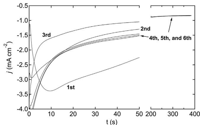
**Fig. 1.** Chronoamperograms of zinc deposition in  $0.34 \text{ mol kg}^{-1} \text{ Zn(TfO)}_2/\text{BMIm TfO}$  within the USAXS electrochemical cell at an estimated overpotential of  $370 \text{ mV}$ . The total charge passed for the 1st, 2nd, and 3rd potential steps was  $400 \text{ Zn ML}$  ( $209.2 \text{ mC cm}^{-2}$ ) and for the 4th, 5th, and 6th potential steps was  $800 \text{ Zn ML}$  ( $418.4 \text{ mC cm}^{-2}$ ).
