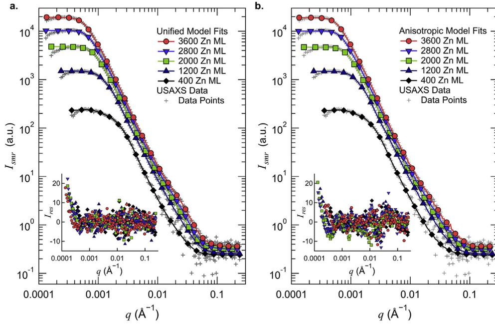
**Fig. 11.** The (a) unified model and (b) anisotropic model fits to the slit smeared USAXS intensity collected for the USAXS scans made after 400, 1200, 2000, 2800, and 3600 Zn ML of charge passed. The normalized residuals for the model fits is shown in the inset graphs within (a) and (b).
